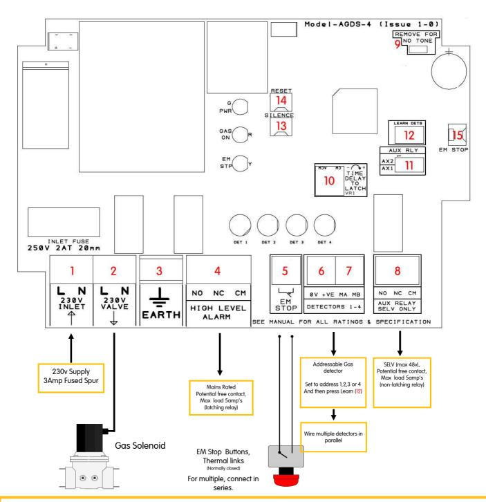
All current wiring regulations must be followed with reference to running low and mains voltage cables together.
