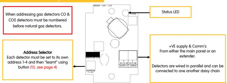
All current wiring regulations must be followed with reference to running low and mains voltage cables together.
