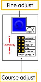
There is a fine adjustment using the potentiometer labelled "Gain" and a coarse adjustment by means of jumper links.
