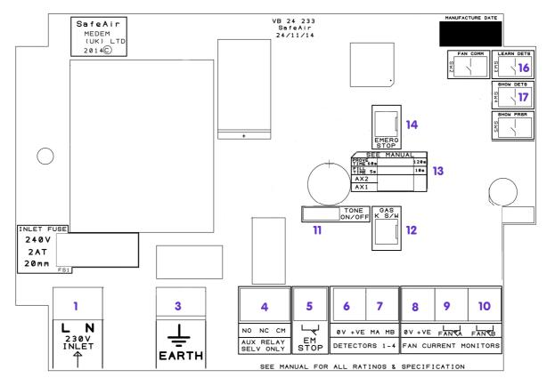
Connections to panel: marked on board.
